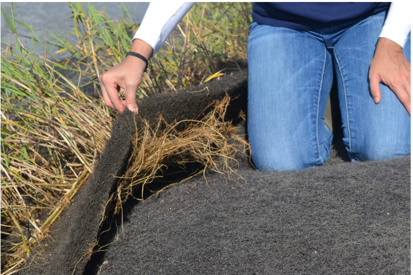
Lifting up of one layer of EcoShield to unveil roots of plants below. Courtesy America's WETLAND Foundation.
