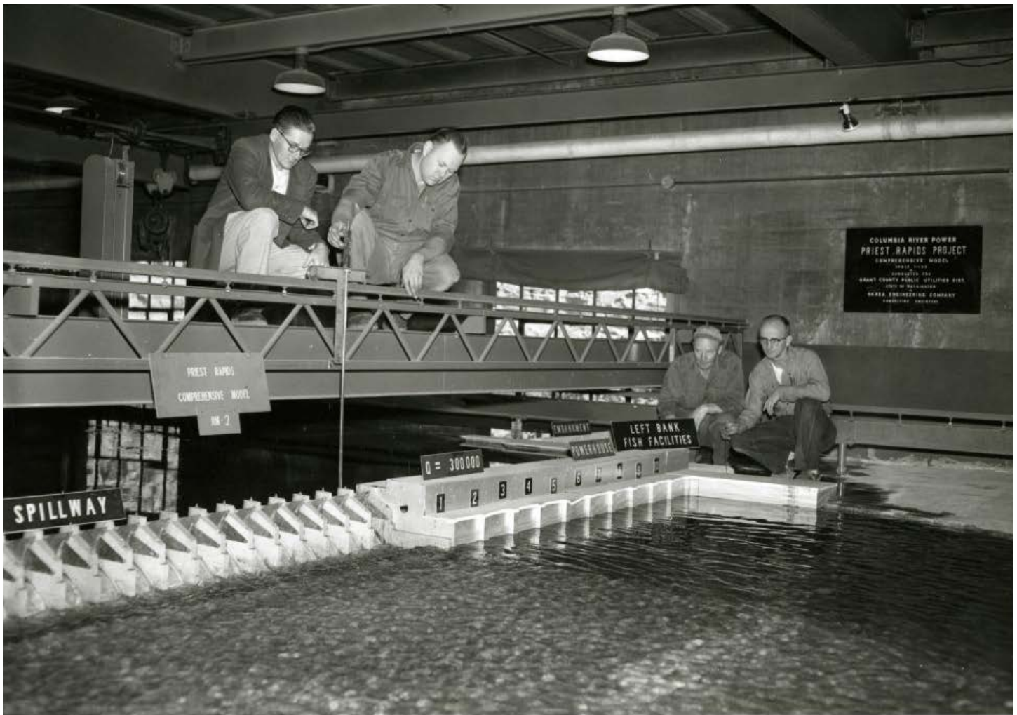
SAFL researchers take measurements of the Priest Rapids physical model. The dam was constructed on the Columbia River in 1961. Image courtesy of SAFL.
