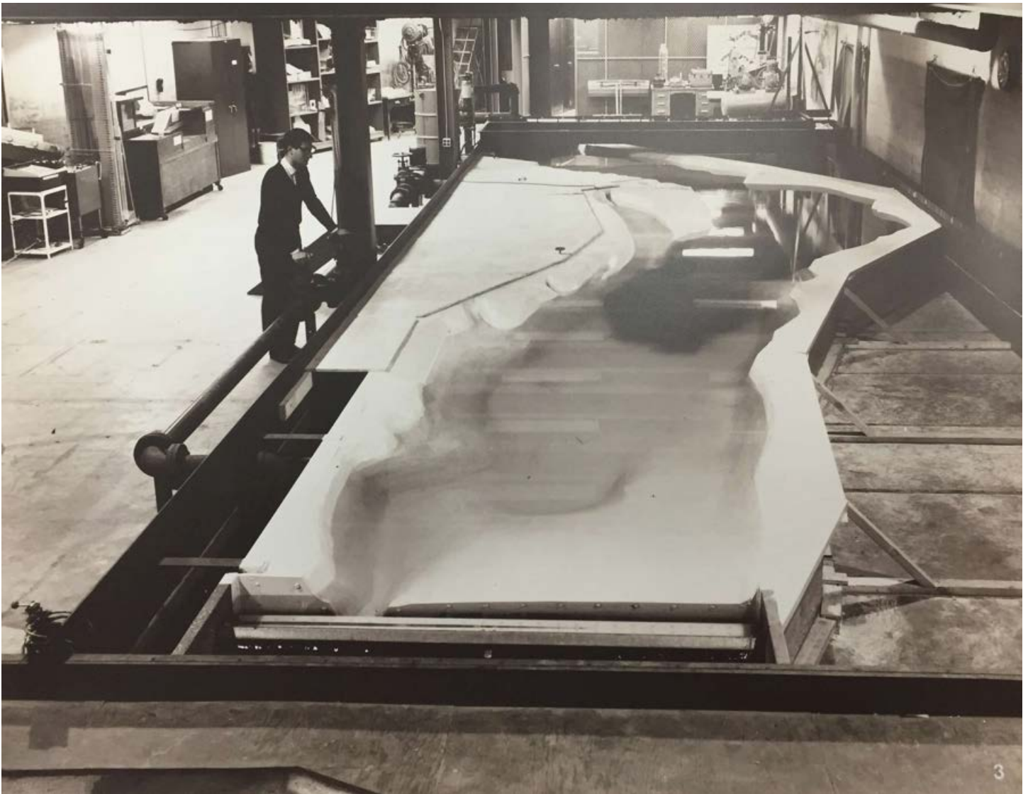
Physical model of the Lake St. Croix. Image courtesy of SAFL.
