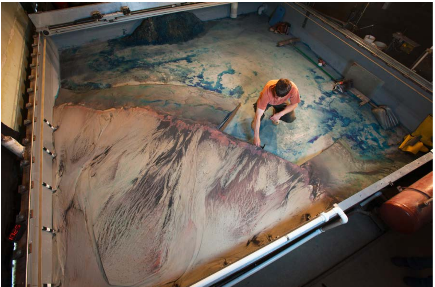
A SAFL student cuts into an experimental delta, revealing the stratigraphy of the deposits. Image courtesy of SAFL.
