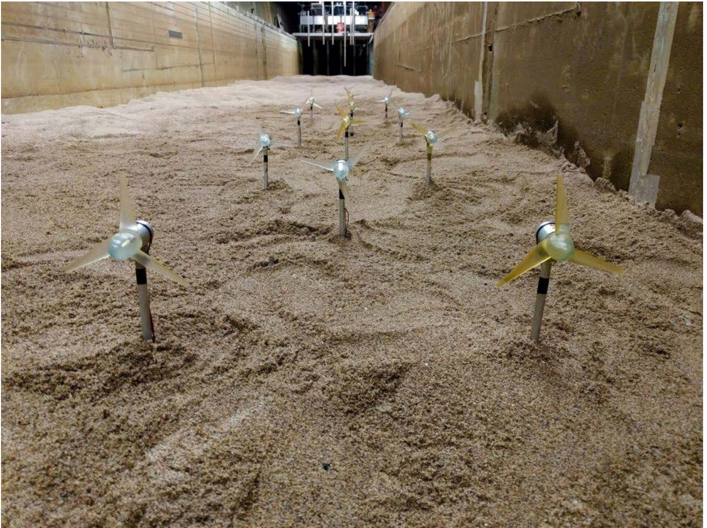
MHK model turbines are set in an array in SAFL's main channel for an experimental run. Image courtesy of SAFL.
