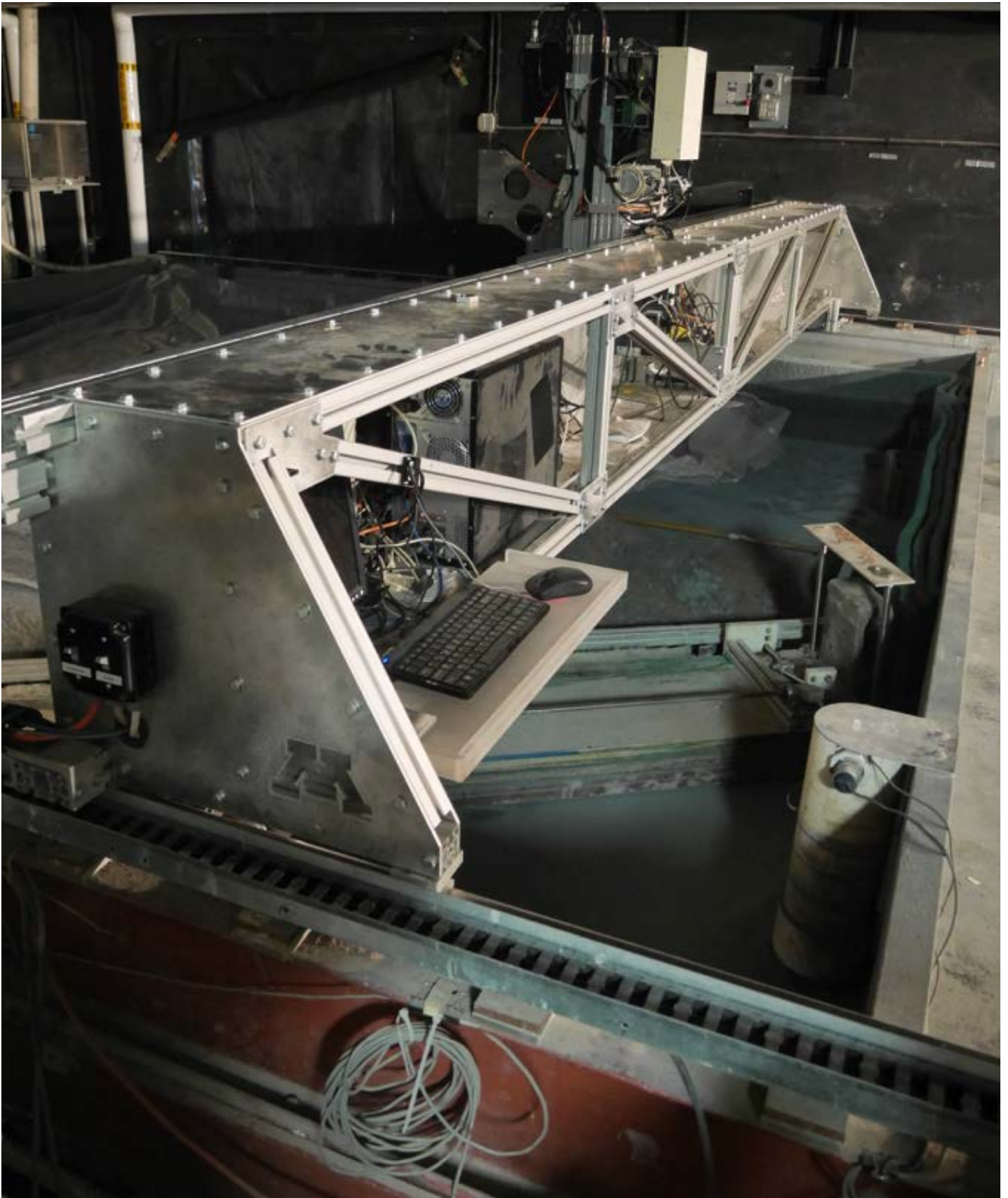
One of SAFL's data collection carriage systems. Image courtesy of SAFL.
