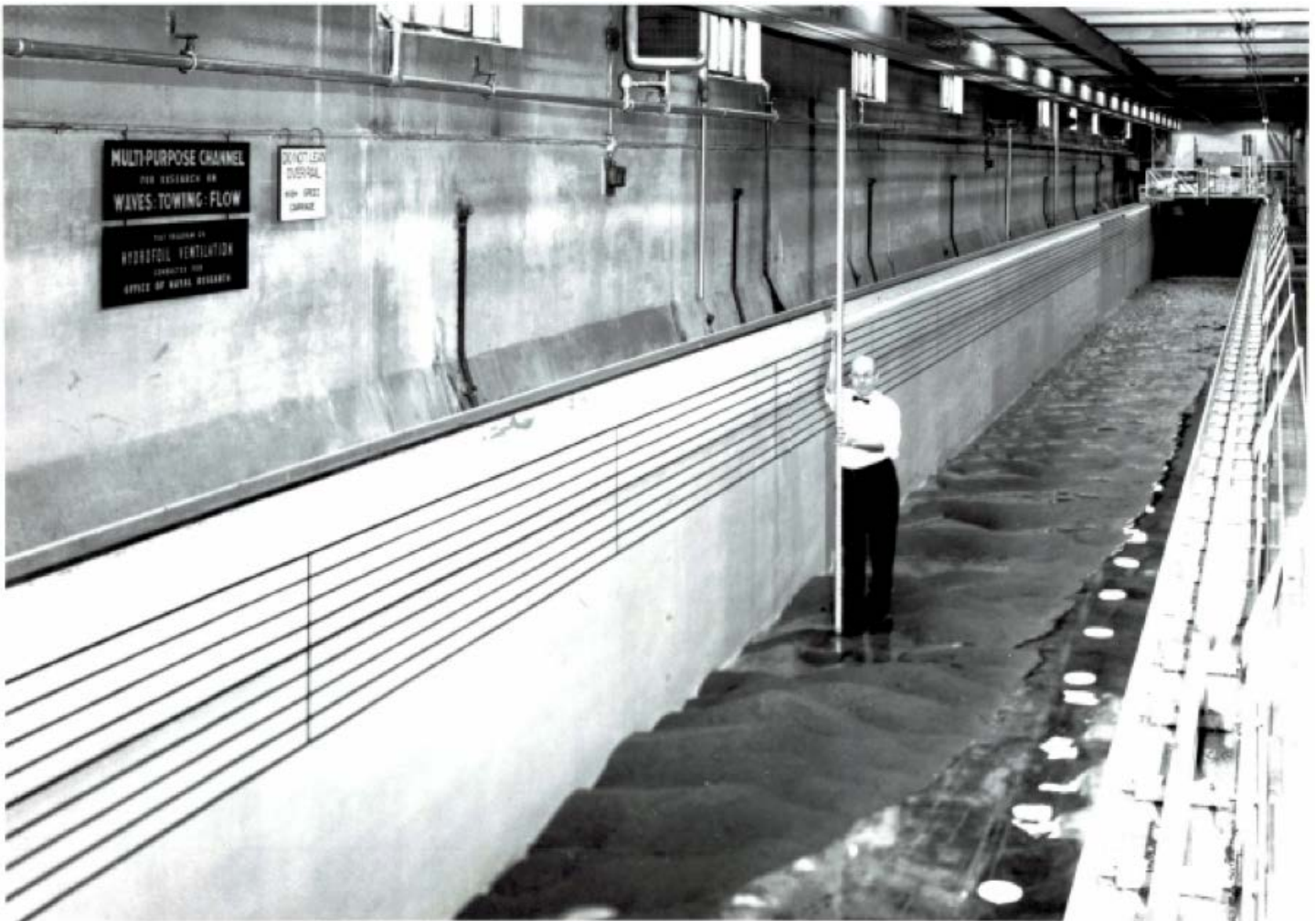
SAFL's Main Channel Flume, which extends the entire length of one floor and can run up to 300 cfs. See sediment transport in this flume in the video included below. Image courtesy of SAFL.
