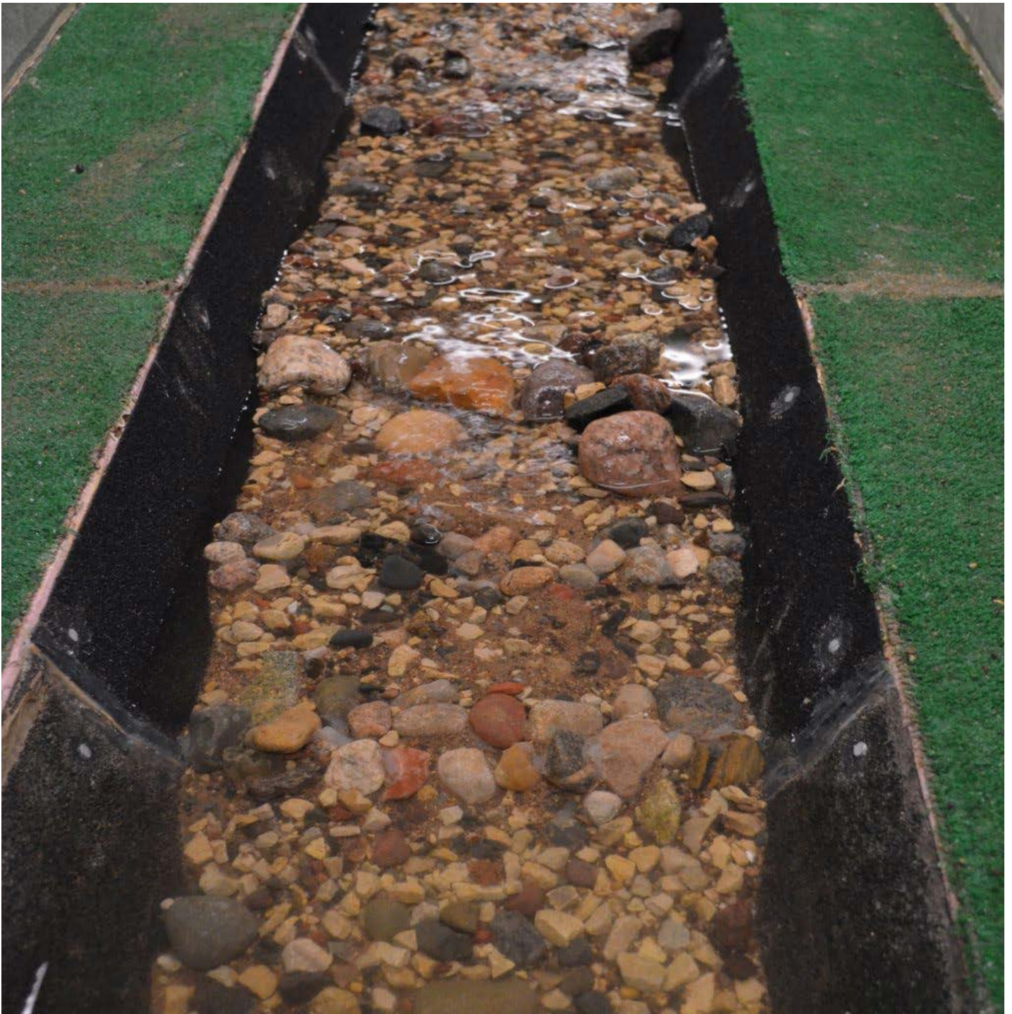
Experimental set up exploring sediment transport dynamics through culverts. Image courtesy of SAFL.
