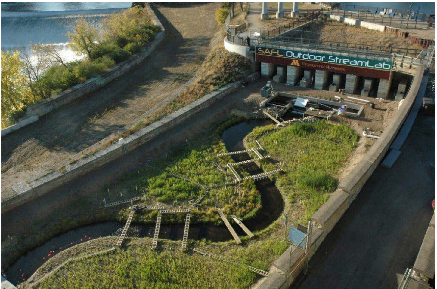
The Outdoor StreamLab (OSL) facility bridges the gap between laboratory and field by allowing control of several parameters (flow, sediment, data collection) while also allowing natural sunlight to drive natural ecological processes. Image courtesy of SAFL.
