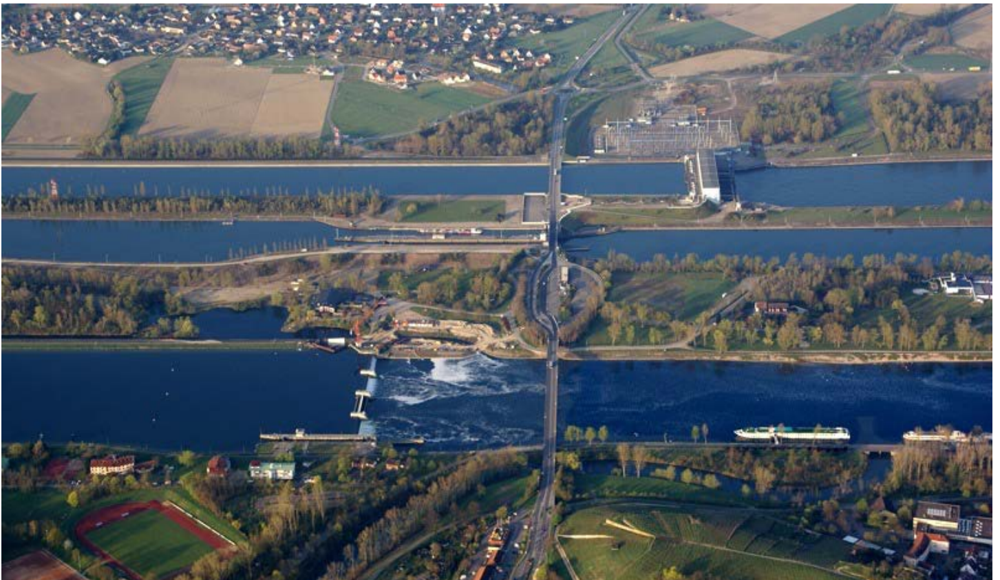
From the bottom of the image to the top: Rhine Canal, navigation channel, hydroelectric plant. Breisach, Germany. Photographer Norbert Blau. Used under Creative Commons (CC BY-SA 3.0).
