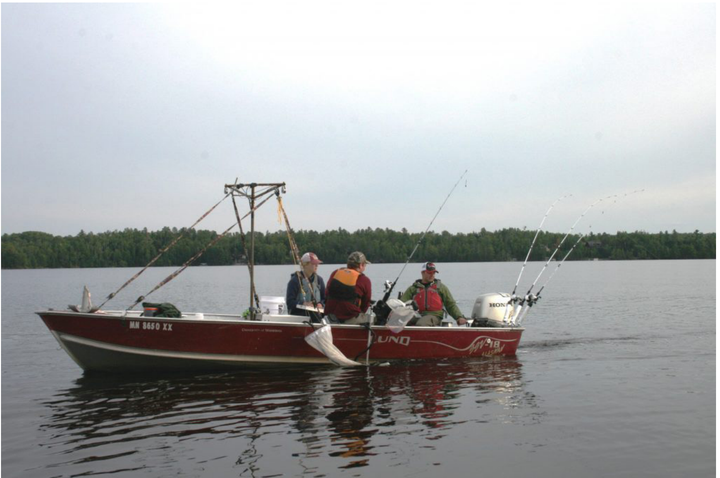
NRRI researchers on Island Lake in northern Minnesota test three different types of fishing line, buoys holding anchor lines and a downrigger to see if spiny water fleas attach to them. Image courtesy of the author.
