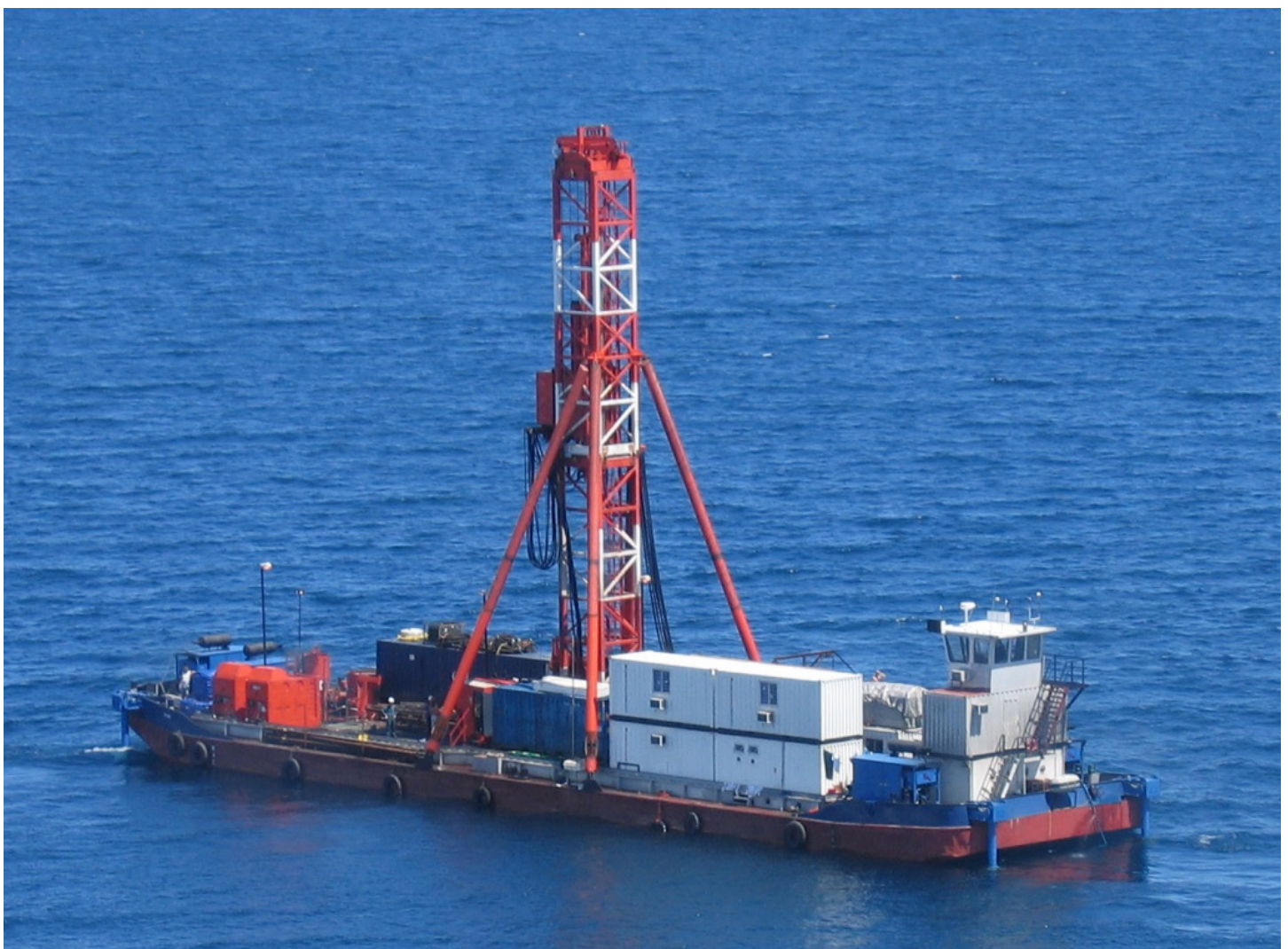
Figure 4. Aerial view of the 160' drilling barge Viphya on Lake Malawi, where 26 members of the drill team, science team, and ship's crew lived for six weeks. This fuel barge was converted to accommodate a 100 ton geotechnical drilling rig (capable of recovering sediment from >1 km below lake surface) and a dynamic positioning system to maintain the position of the drilling barge in waters too deep for anchoring. Photo credit: Isla Casteneda.
