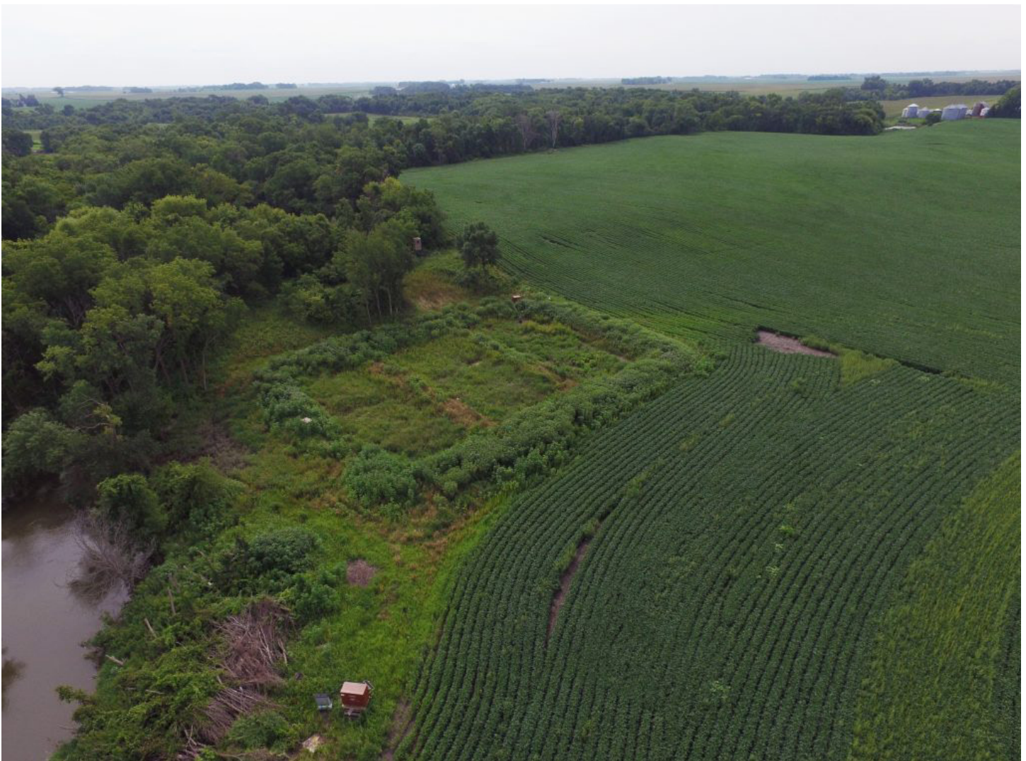
A three-cell treatment wetland on a Martin county farm removes nitrogen and phosphorus from tile drainage before it flows into Elm Creek. Image courtesy of David Hansen.
