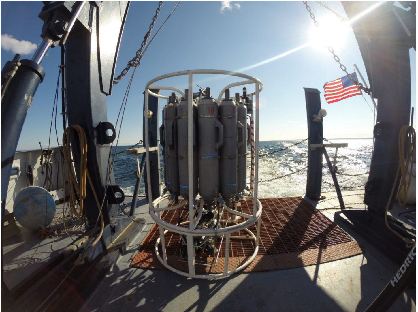
Figure 1. The bottom of Lake Superior is below sea level! To measure certain parameters and to collect water from hundreds of meters below the surface, scientists can deploy this “CTD rosette.” The gray vertical tubes are water sampling bottles that can be closed at chosen depths so that water from that location is brought back on board. Below the gray tubes is a package of instruments that measures such things as temperature, salinity, oxygen, and other parameters, giving LLO scientists a “vertical profile” of lake conditions. Photo credit: Blue Heron crew.
