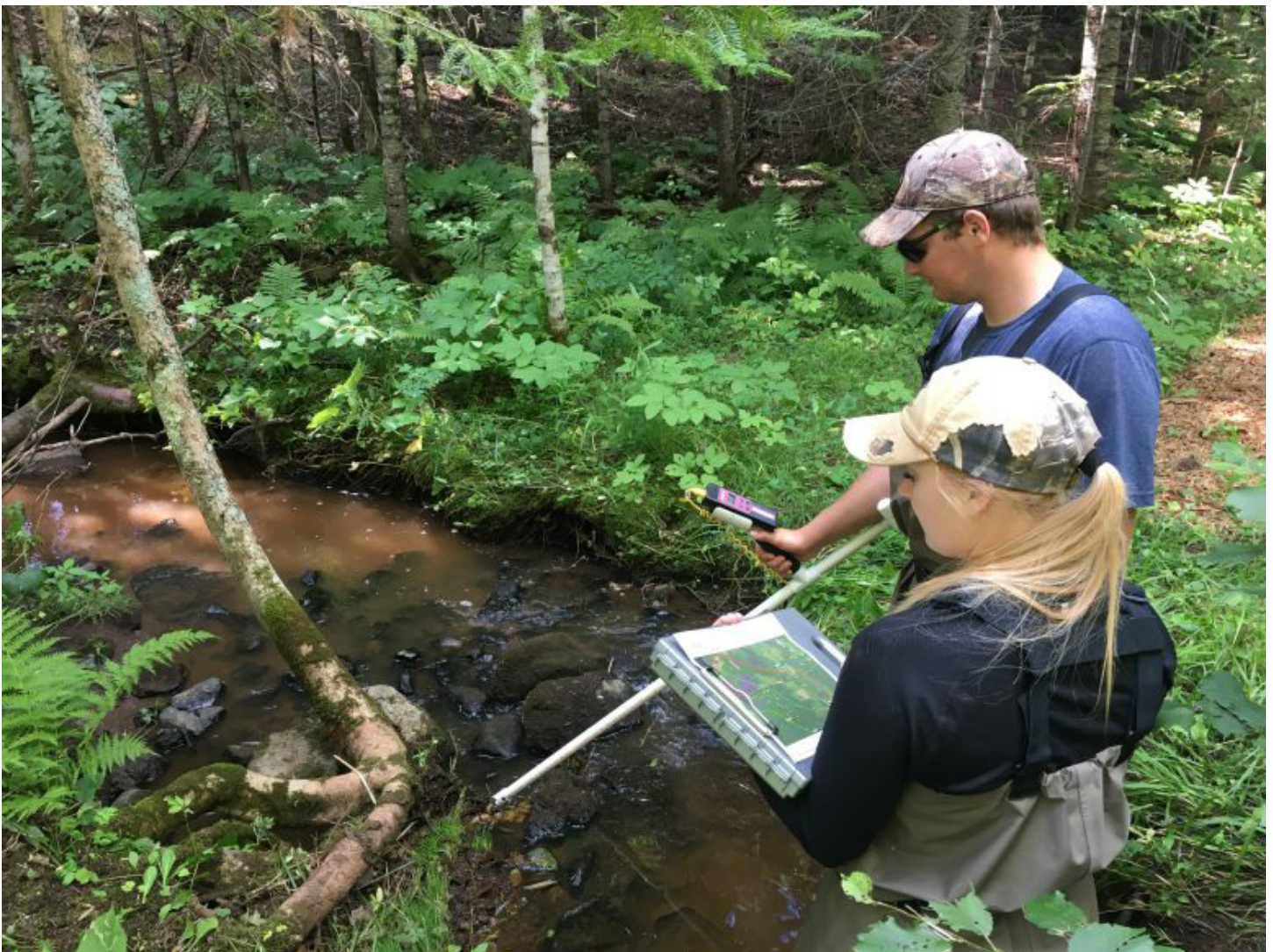
NRRI Field Technicians Nick Pierce and Kari Hansen walk through rural streams to get temperature readings, documenting where cool water inputs might make them more resilient against climate change impacts. Image courtesy of the author.
