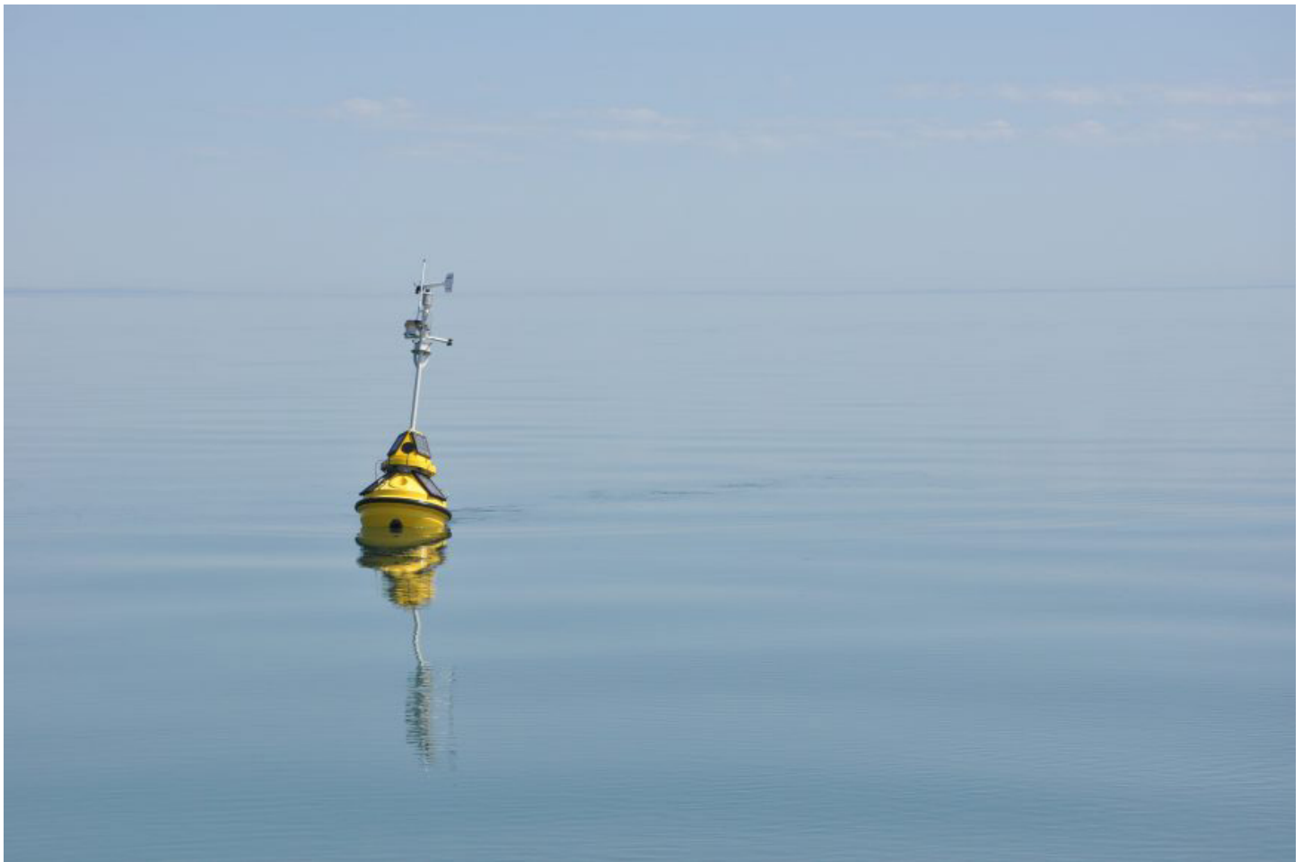
Figure 8. One of LLO’s solar-powered buoys on a calm, sunny Lake Superior day, sending data concerning air and water conditions to shore. During the open water season, data from LLO’s two buoys (LLO1 and LLO2) are available from http://d.umn.edu/buoys/ .
