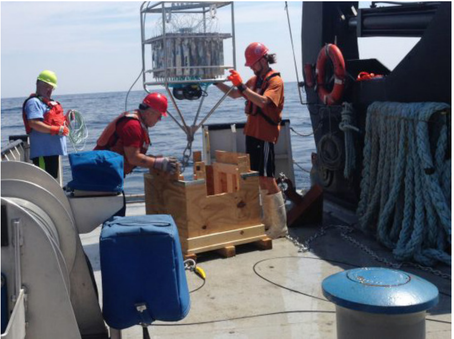
Deploying one of the buoy systems with remote sampling devices to collect year-round data on the Great Lakes. Image courtesy of Euan Reavie.
