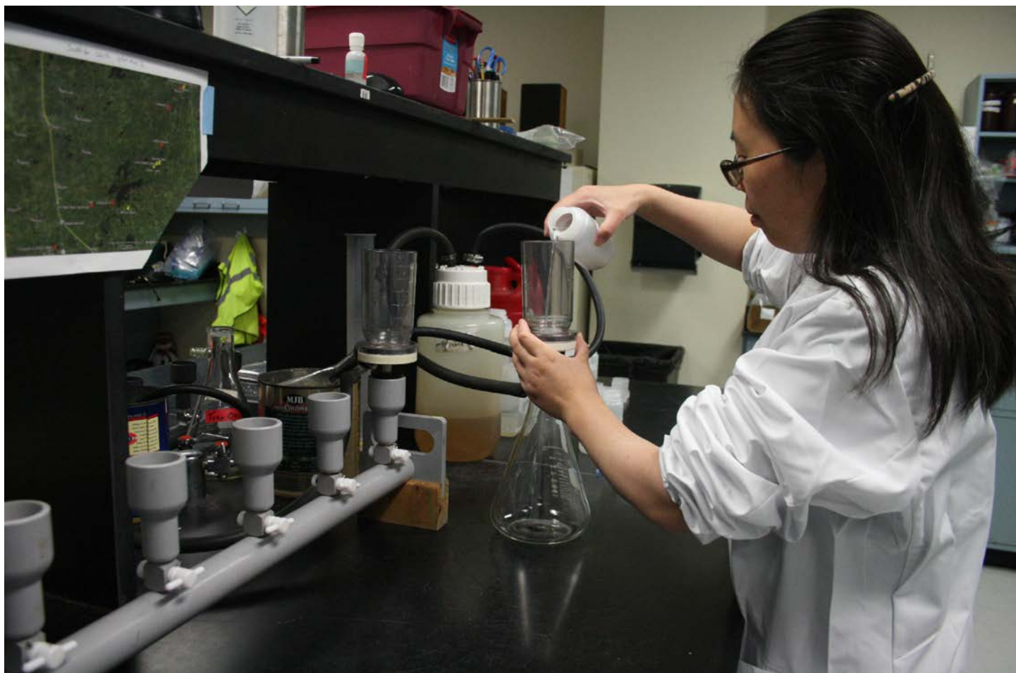
NRRI Researcher Meijun Cai filters water in her lab as part of an experiment to use local waste resources to remove pollutants from road runoff. Image courtesy of the author.
