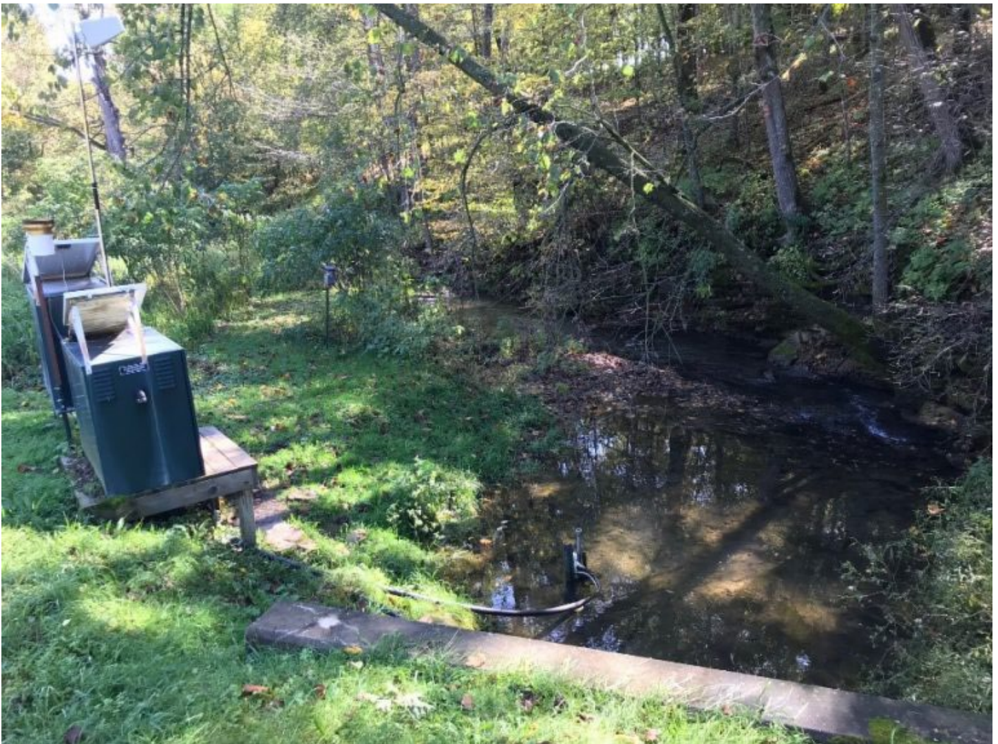
In-stream monitoring stations were installed at the outlets of the small study watersheds. This information combined with edge-of-field monitoring and a wide range of other assessments provides a unique opportunity to evaluate the effects of targeted agricultural conservation practices on water quality. Image courtesy of Kevin Kuehner, Minnesota Department of Agriculture.
