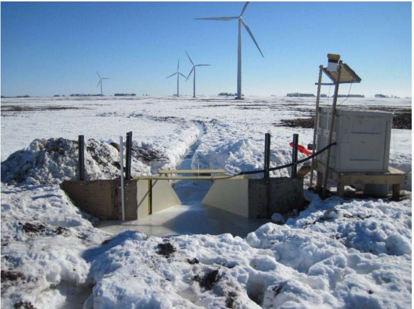
Edge-of-field monitoring stations provide information about the amount of runoff, soil, and nutrients moving off a given field into the waterway. Sites are fully automated to collect water samples whenever runoff occurs. Water samples are analyzed for nitrogen, phosphorus, and sediment and monitoring occurs year-round, 365 days a year. Monitoring has shown that 40 percent of the surface runoff occurs when the ground is frozen. Image courtesy of Kevin Kuehner, Minnesota Department of Agriculture.
